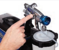
2) Slide trigger lever to release needle
