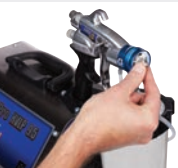
1) Remove front air cap and nozzle
