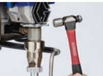
1) Loosen the clamping nut
